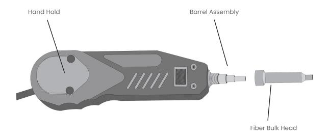
Locate the bulkhead you want to install and look to the threaded end. This screw acts as a "key" and is already mounted with the key channel. Do not try to screw the key channel from the threaded key, which might cause damage to the probe installed.
